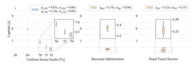
Figure 28: Lap times across 10 laps with the proposed *ForzaETH Race Stack* using the MAP controller. Uniform sector scalers in blue, BO obtained sector scalers in green, and hand-tuned sector scalers in bronze. The mean and standard deviation of all corresponding lap times are depicted in the top right, zoom in to enhance visibility when necessary.
