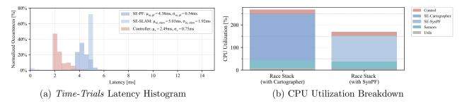
Figure 31: Latency histogram and CPU utilization breakdown of the ForzaETH Race Stack during the Time-Trials phase. Latencies of the Control module are obtained from the run with Cartographer-SLAM.
