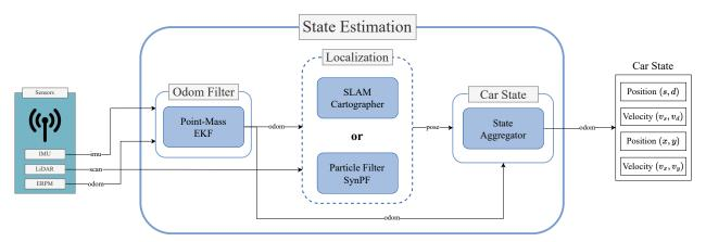
Figure 5: An overview of the proposed state estimation system architecture. The state estimation module incorporates velocity estimation and localization with respect to the pre-mapped racetrack and aggregates this information in a final car state odometry output both in Cartesian and in *Frenet* coordinates.
