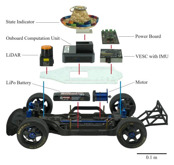
Figure 2: Comprehensive overview of the autonomous racing platform's hardware architecture. This figure presents an exploded view of the racecar, highlighting its key components as well as their integration.
