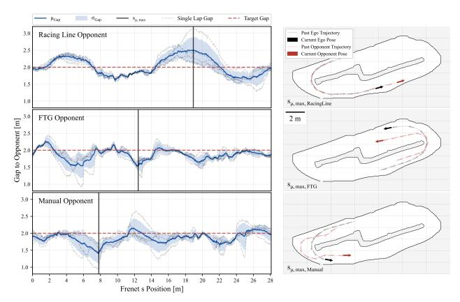
Figure 25: Trailing gap over four consecutive laps against three different opponents is shown. The reference gap is depicted in red, the mean and standard deviation from the reference gap in blue, and the measurements of the gap in each lap in grey.
