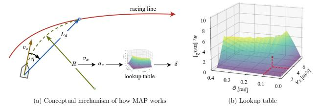
Figure 23: (a) MAP obtains required centripetal acceleration  $a_c$  to reach a lookahead point  $L_d$  using the  $L_1$  guidance law. (b) The lookup table is used to retrieve the steering angle  $\delta$  that results in the calculated  $a_c$  for the speed  $v_x$ .
