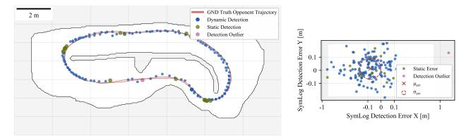
Figure 12: Evaluation of the spatio-temporal detection accuracy during multiple laps on a track, by trailing behind an opponent with the perception system active. Left: Spatial detections (blue), opponent trajectory (red), static detections (green), and detection outliers (purple). Right: Detection error in a symmetric linear-logarithmic plot; shaded regions indicate logarithmic scales and purple marks are outliers excluded from the RMSE calculation.
