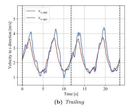
Figure 24: Velocity data over two consecutive laps, on the left the car is driving in the state *GBFree* and on the right trailing an opponent. The to-be-tracked reference velocity is the velocity of the global waypoints in the state *GBFree* and the opponent's velocity in the state *Trailing*. The start of a new lap is marked by the black dashed line.
