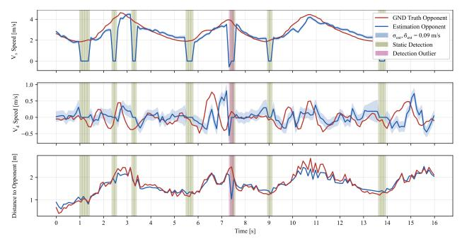
Figure 13: Opponent velocity estimation associated to the detections in Fig. 12. Ground-truth measurements of the opponent states are depicted in red, while the velocity estimation of the opponent is highlighted in blue. Green-shaded regions are static classifications of the opponent. Purple-shaded regions depict detection outliers, i.e. exceeding an error of twice the measurement standard deviation.
