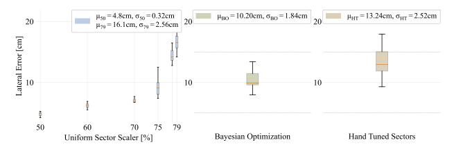
Figure 29: Lateral error across 10 laps, relative to the optimal racing line using the *ForzaETH Race Stack* with the MAP controller. Uniform sector scalers (blue), BO scalers (green), and hand-tuned scalers (bronze). The mean and standard deviation are in the top right.
