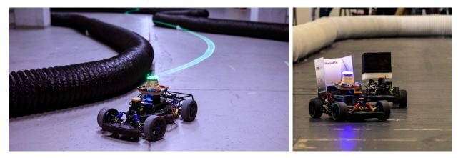
Figure 1: The physical ForzaETH autonomous racecar running the proposed ForzaETH Race Stack. On the right, an overtaking maneuver during the ICRA23 F1TENTH race.
