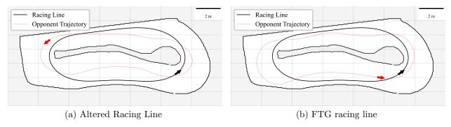
Figure 32: Opponent Racing Lines for the *Head-to-Head* analysis. The altered racing line was obtained by modifying the boundaries and then applying the minimum curvature racing line optimizer discussed in Section 6.2, while the FTG racing line is a result of the algorithm as described in Section 8.1.
