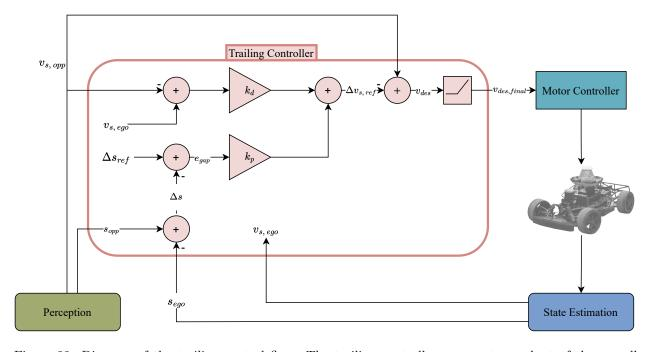
Figure 22: Diagram of the trailing control flow. The trailing controller represents a subset of the overall *Control* module of Fig. 21. It is responsible for maintaining a close and steady distance towards the opponent while avoiding collisions. This allows the agent to set itself up well for a possible overtaking maneuver.
