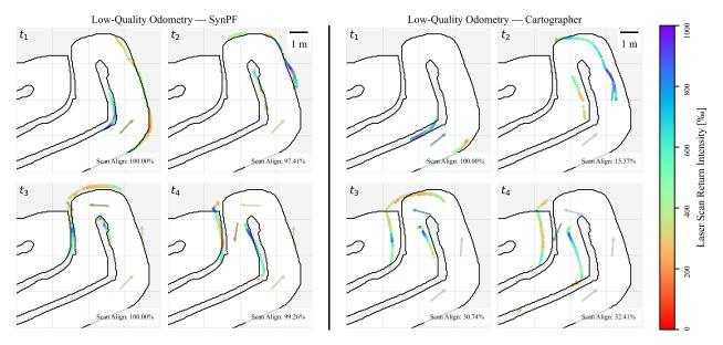
Figure 7: Low-quality odometry conditions corresponding to the right-hand side of Fig. 6 showcasing both Cartographer and SynPF under worst-case conditions in four sequential time steps, indicated with  $t_i$ . At  $t_2$ , Cartographer is unable to align the LiDAR scans with the track boundaries, while SynPF maintains a visibly steady track alignment.
