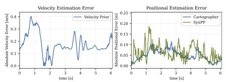
Figure 10: State estimation error curves for cartesian coordinates and longitudinal velocity corresponding to one lap around the test track. Where relevant, the two different localization techniques available are compared against ground-truth data, and the velocity and positional error are depicted for the duration of a single lap.
