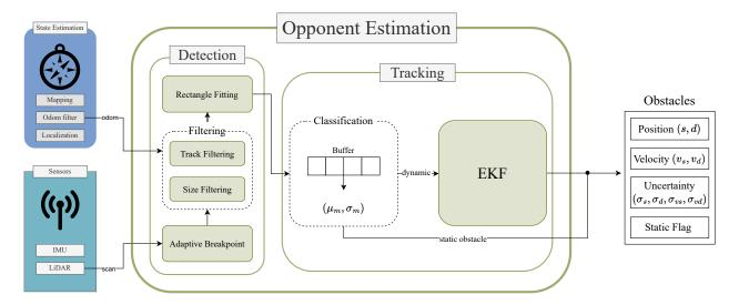
Figure 11: Overview of the proposed opponent estimation system architecture. The opponent estimation module incorporates the detection and tracking submodules and is integrated into the *ForzaETH Race Stack*, as depicted in Fig. 3.
