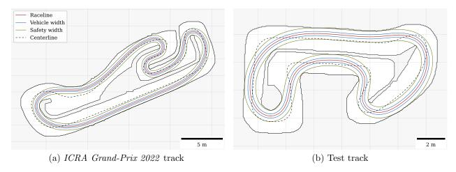
Figure 19: The global trajectory optimized with iterative minimum curvature on two different tracks. Besides the racing line (red), the figure also shows the centerline (dashed black) and the vehicle width without (blue) and with a safety distance (green). The illustration shows that even with the conservative safety distance the selected optimizer finds a feasible trajectory for typical F1TENTH competition tracks.
