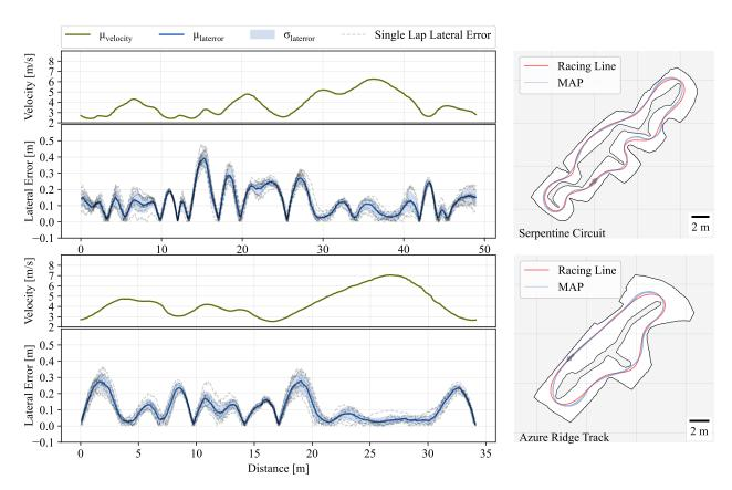
Figure 26: Ten laps of the MAP controller on two different real-world tracks tracking a reference racing line. The left side shows velocity and average and per lap lateral tracking error. On the right, the map and trajectories of the laps are shown.
