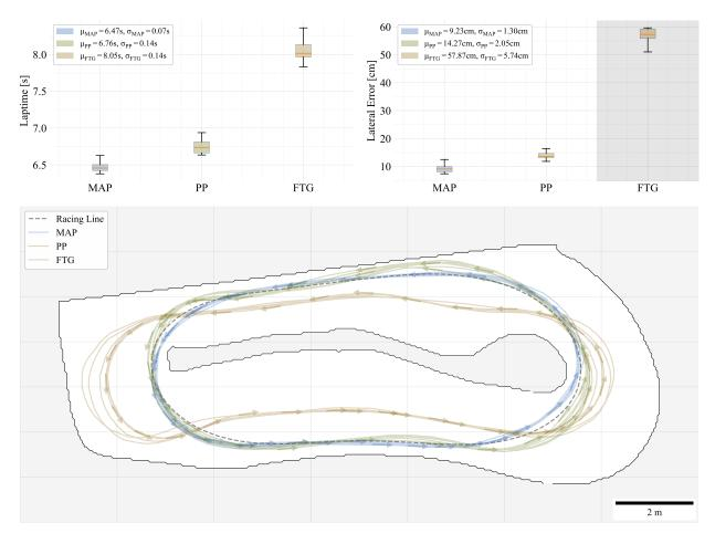
Figure 30: A lap time and lateral deviation comparison of the proposed ForzaETH Race Stack configuration against a different controller configuration of the race stack and a completely reactive FTG race stack. MAP denotes the proposed configuration, PP denotes a popular alternative for autonomous racing, and a fully reactive FTG race stack that does not adhere to the See-Think-Act cycle.
