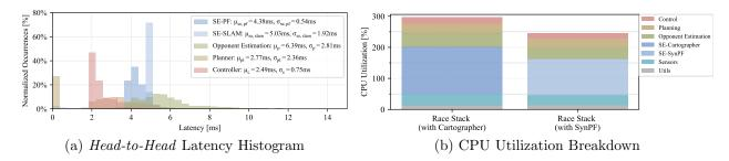
Figure 33: Latency histogram and CPU utilization breakdown of the ForzaETH Race Stack during the Head-to-Head phase. Latencies of the Opponent Estimation, Planning, and Control module are obtained from the run with Cartographer-SLAM.
