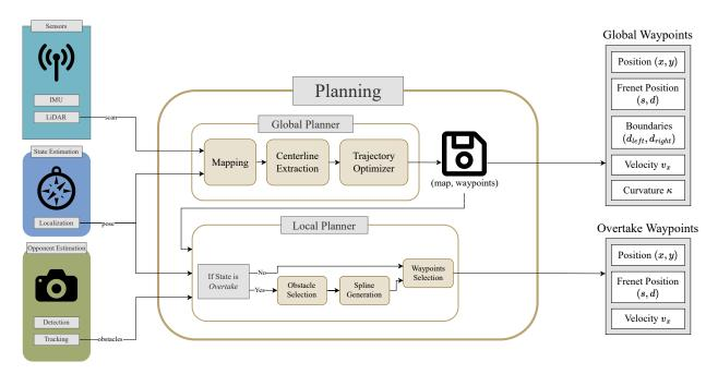
Figure 14: Overview of the proposed planning module. The system integrates a global planning submodule for computing an optimal racing line offline, alongside a local planner that dynamically responds to opponent estimations to compute overtaking trajectories.
