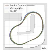
Figure 9: On the small racetrack set up with the motion capture system, *Car*tographer is able to closely match the ground-truth trajectory, while *SynPF* performs slightly worse.
