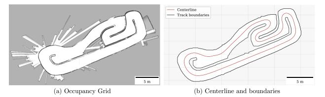
Figure 15: The centerline extraction step of the global planner shown on the track of the *ICRA Grand-Prix* 2022. Fig. 15a: Occupancy grid obtained by SLAM. Fig. 15b: Extracted centerline (red) including track boundaries (black).
