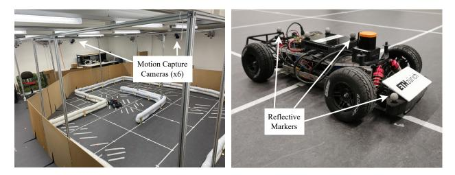
Figure 8: Experimental setup with the motion capture system and mounted reflective markers.
