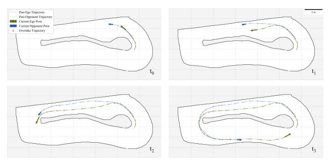
Figure 20: Sequential frames of an overtaking maneuver. The blue trajectory represents the opponent, while the green trajectory is that of the ego-agent. The figure also shows the ego and opponent poses, and the planned overtaking waypoints for each timestep. It can be seen that in the frames after the overtake has happened  $(t_2, t_3)$  the planned waypoints are on the nominal racing line.
